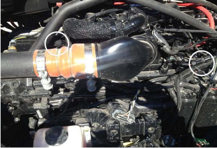
**2)** Unplug both sets of stock injector connectors. Press the release tab on the connector and gently pull the connector apart.
