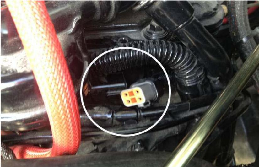
3) Route the module harness as shown in the picture below. The module case will be located closer to the Flywheel side of the engine.
