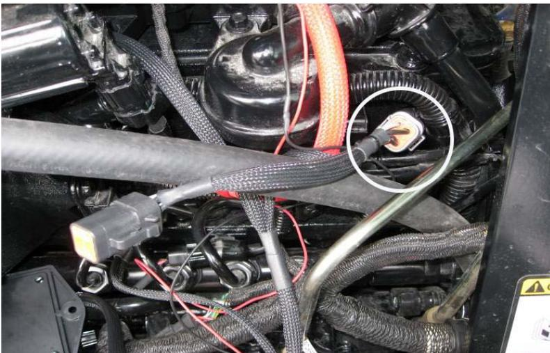
**5)** On the Ag Diesel Solutions harness, the male injector connector located closest to the module case will connect to the female injector connector located closest to the Flywheel-side of the engine.
